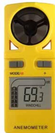
*Figure 11.5: Using an anemometer to check wind speed at roof level.*
