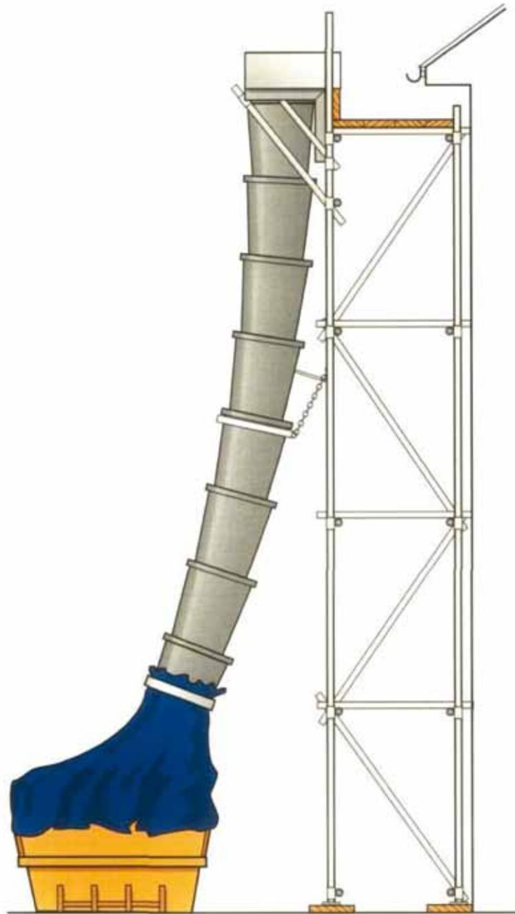
*Figure 11.7: Waste chutes make waste handling easier and safer.*
